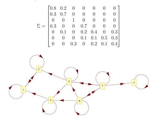
Figure 3: The network  $\Sigma$  in matrix notation and the associated graph.
